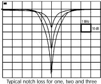
cavity assemblies for 3 dB bandwidth = 3 MHz.
