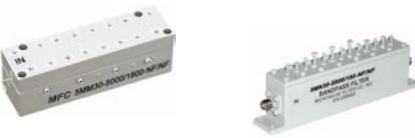
Microwave Filter Company's Iris coupled, Combline and Interdigital bandpass filters are fixed tuned filters that feature sharp stopband rejection and lower losses than comparable discrete element or tubular (transmission line) bandpass filters. Parallel coupled, distributed round rod resonators provide high-Q with small size and excellent bandpass response.
