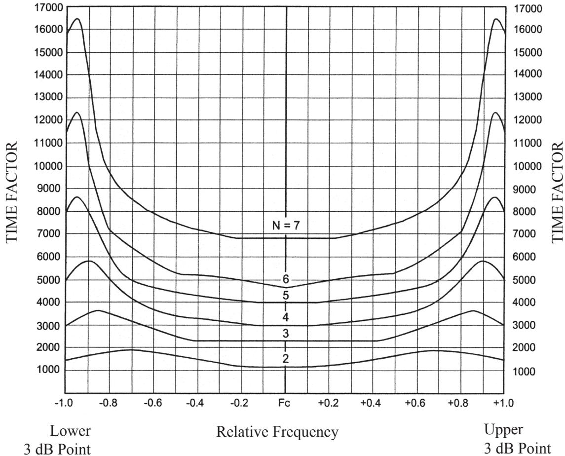
The approximate group (time) delay of an MFC Chebyshev bandpass filter can be calculated using the following equation:
