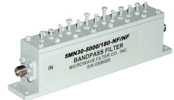
Microwave Filter Company's Iris coupled, Compline and Interdigital bandpass filters are fixed tuned filters that feature sharp stopband rejection and lower losses than comparable discrete element or tubular (transmission line) bandpass filters. Parallel coupled, distributed round rod resonators provide high-Q with small size and excellent bandpass response.
