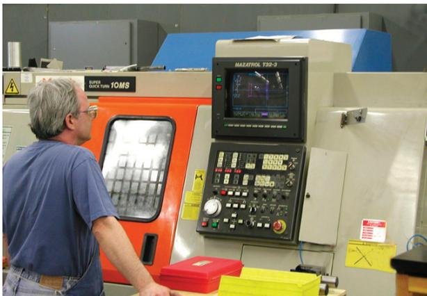
Mazak CNC Lathe for Production Prototyping
